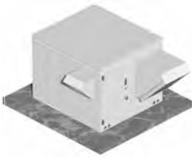
Foundation Mounting for Arr. H
