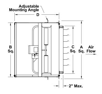
Note: Correct propeller rotation is CCW when viewing from inlet side.
